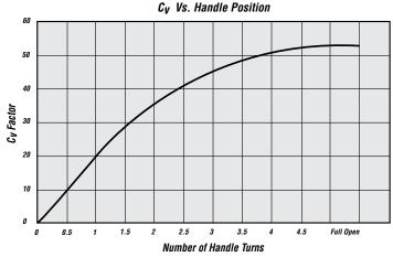
Test Media: Deionized Water @ Room Temperature Port Size: 2"
