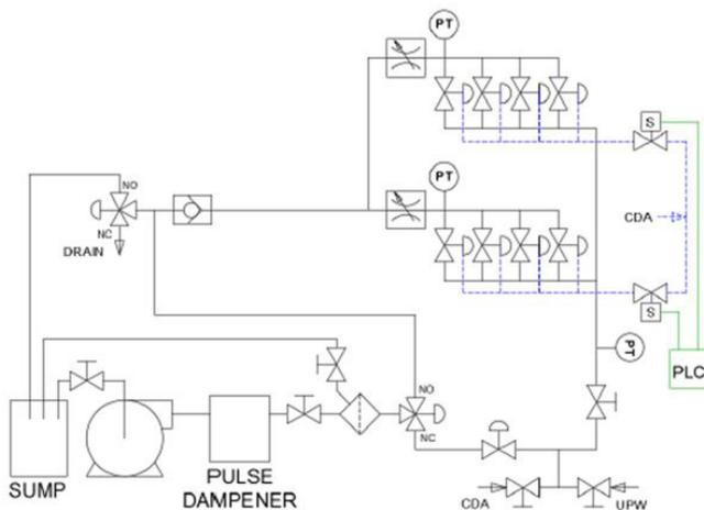
The accelerated life test was performed on a set of eight valves in 49% HF. Cleanroom grade HF was used. The acid was replaced halfway through the test to ensure that full chemical strength was maintained.
